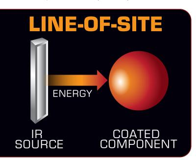
Since most automotive components are quite adept at conducting heat, energy may be passed along the substrate, curing areas out of direct IR line-of-sight. Heat resulting from IR energy may also provide a degree of convection heating, which also helps to achieve non line-of-sight curing. However, these are poor substitutes for direct line-of-sight IR curing.
